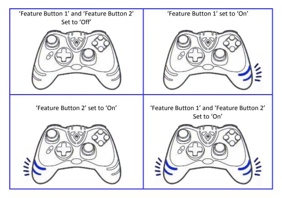
**TurboFire and WildFire Wireless Controller:** The feature indicator light will only illuminate on the left handle of the pad when the 'Feature Button 1' is set to 'On'.
